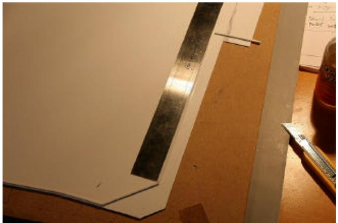
The curbs are made from Evergreen Styrene Strips # 154 (0.06x0.08" / 1½x2mm) and glued on with Plastruct Plastic Weld. I used a steel ruler to make sure they are straight.
